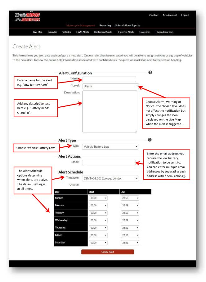
The low battery alert will generate an email when there is approximately 20% capacity left in the vehicle battery, based on a standard lead acid battery.
