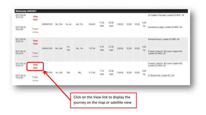
The map view displays the chosen journey with the speed and location recorded every 15 seconds. The display can be toggled from map view to satellite view and you can follow the journey in detail using the on screen arrows. Click on any map marker to view further detail.
